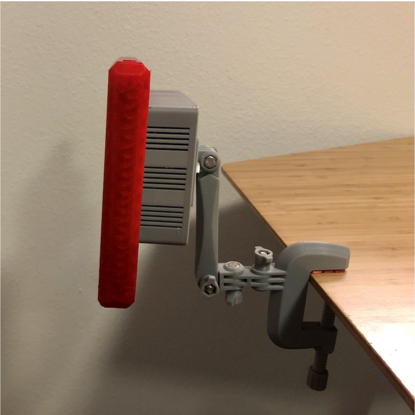
Figure 23a: Our design uses a clamp to attach to tables, bookshelves and other similar surfaces.
